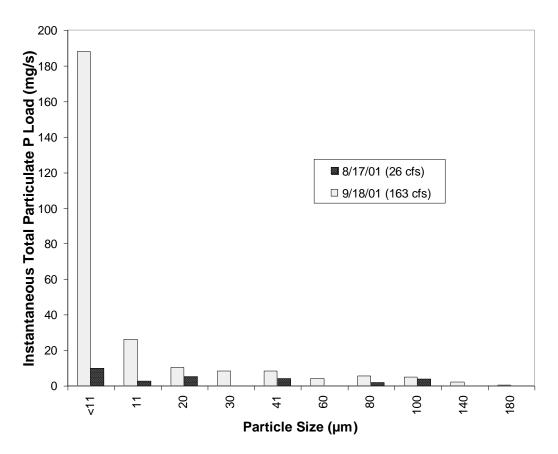
Figure 5. Instantaneous Total Particulate Phosphorus Load by Particle Size.
