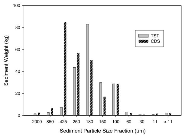
Figure 8. Particle Size Distribution of Suspended Solids Removed from the CDS and TST Units.
