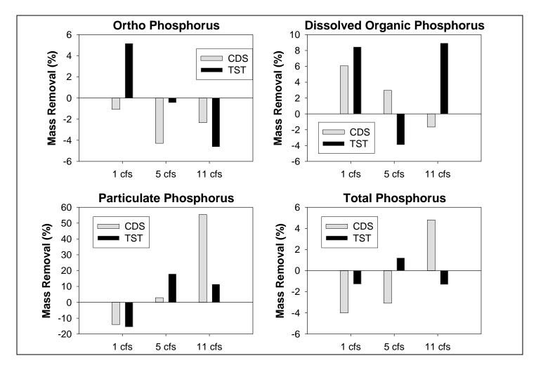
Figure 7. Comparative Mass Removal Efficiencies for Phosphorus Species in the CDS and TST Units.
